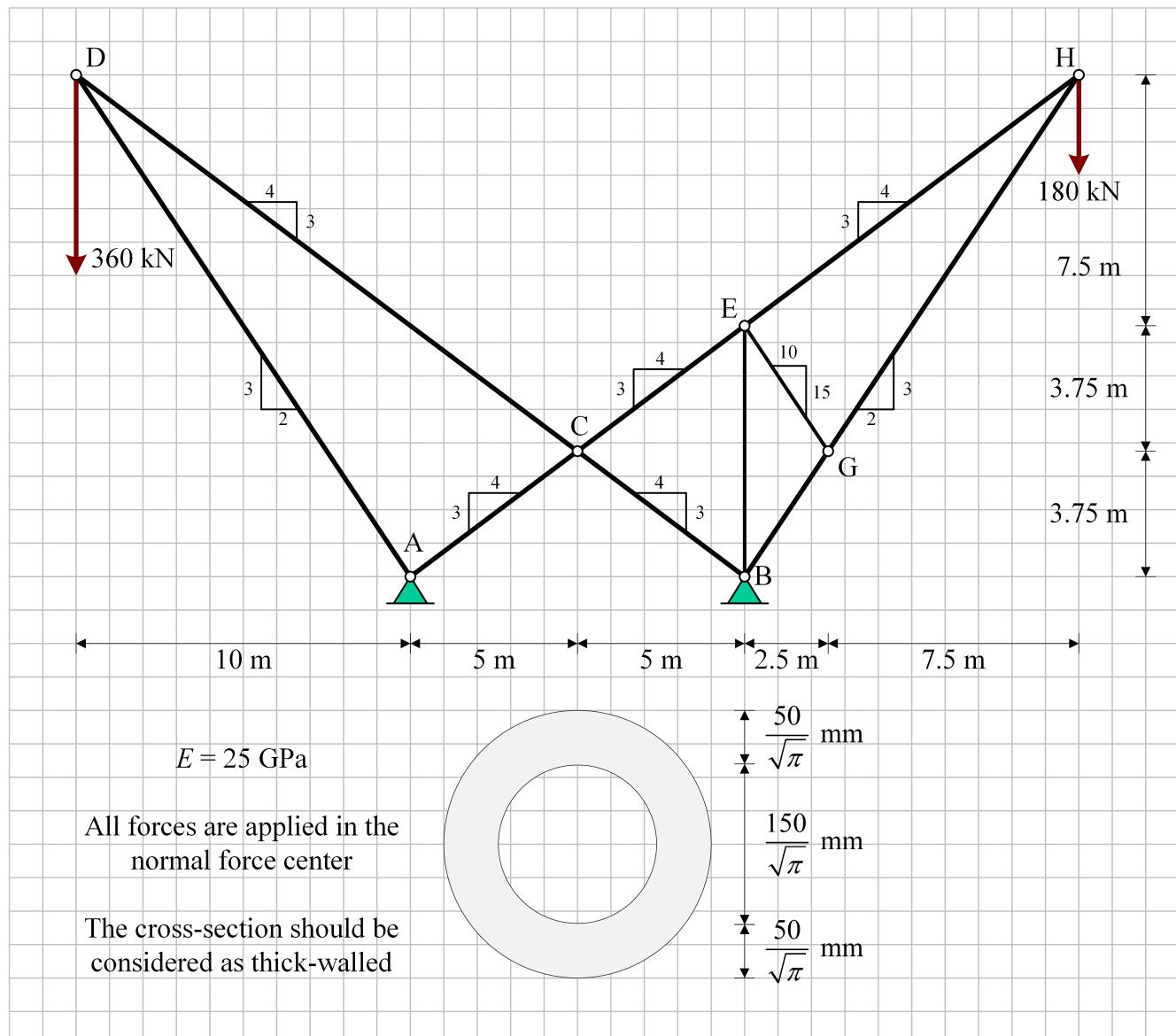
**1a** Determine the normal force in bar CD and AC.
